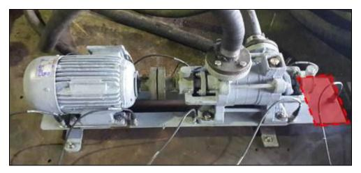
Figure 2. Electric Motor Driven Pump Set-up
