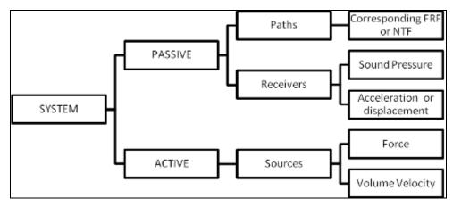
Figure 1. Description of a Mechanical Vibrating System
