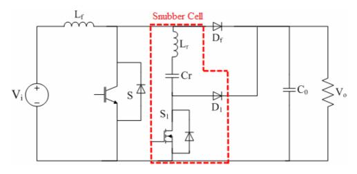
Figure 2. The basic ZCT converter circuit [2]
