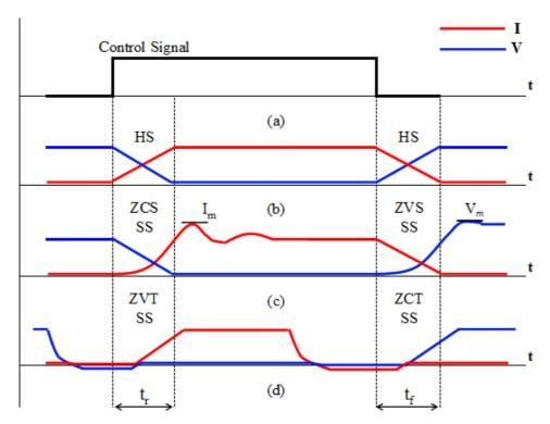
Figure 1. (a) Switching signal, (b) HS, (c) ZCS and ZVS, (d) ZCT and ZVT waveforms
