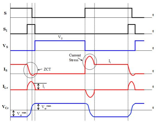
Figure 3. Switching signal of the main switch (S), switching signal of the auxiliary switch (S<sub>1</sub>), the main switch voltage (V<sub>S</sub>), the main switch current (I<sub>S</sub>) and  $L_r$  inductance current (I<sub>Lr</sub>), the voltage of  $C_r$  (V<sub>Cr</sub>) [2].
