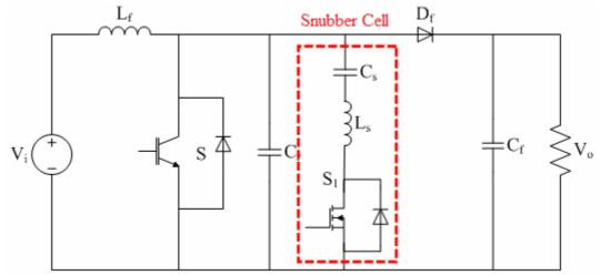
Figure 6. The ZVZCT DC-DC converter [7]
