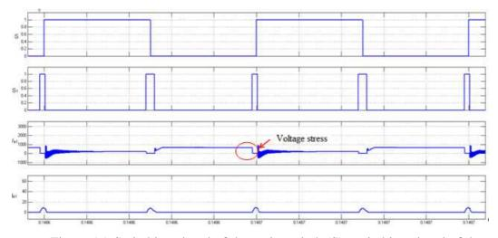
Figure 15. Switching signal of the main switch (S), switching signal of the auxiliary switch ( $S_1$ ), the auxiliary switch voltage ( $V_{S1}$ ) the auxiliary switch current ( $I_s$ )
