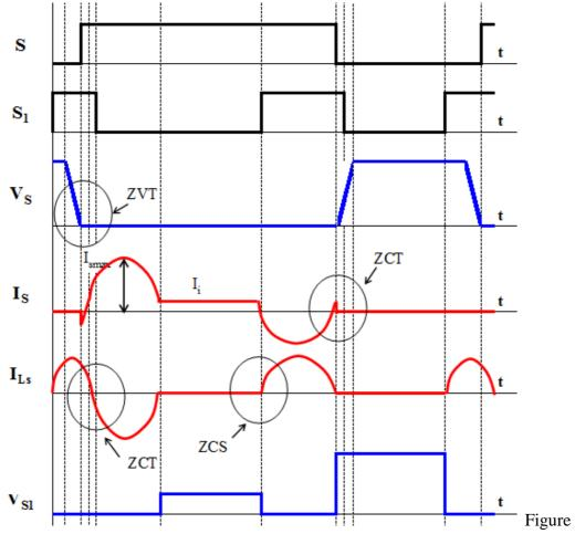
7. Switching signal of the main switch (S), switching signal of the auxiliary switch (S<sub>1</sub>), the main switch voltage (V<sub>S</sub>), the main switch current (I<sub>S</sub>) and L<sub>s</sub> inductance current (I<sub>Ls</sub>), the auxiliary switch voltage (V<sub>S1</sub>) [7]
