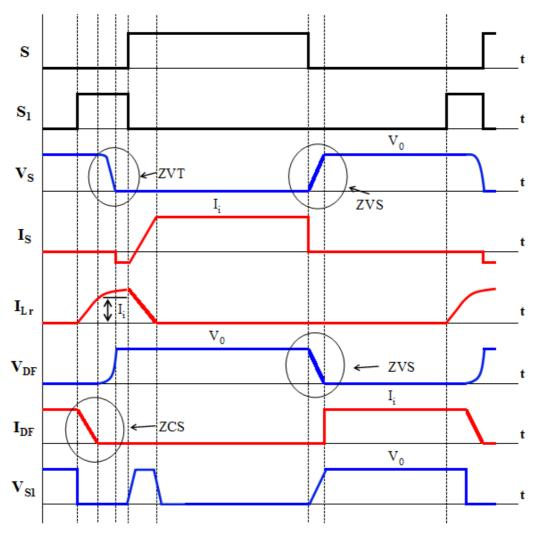
Figure 5. Switching signal of the main switch (S), switching signal of the auxiliary switch (S<sub>1</sub>), the main switch voltage (V<sub>S</sub>), the main switch current (I<sub>S</sub>) and L<sub>r</sub> inductance current (I<sub>Lr</sub>), the main diode voltage (V<sub>DF</sub>), the main diode current (I<sub>DF</sub>), the auxiliary switch voltage (V<sub>S1</sub>) [5]
