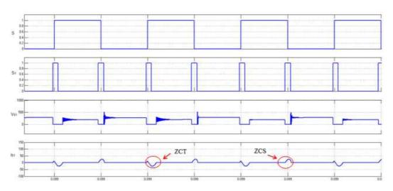
Figure 12. Switching signal of the main switch (S), switching signal of the auxiliary switch ( $S_1$ ), the auxiliary switch voltage ( $V_{S1}$ ) the auxiliary switch current ( $I_S$ )
