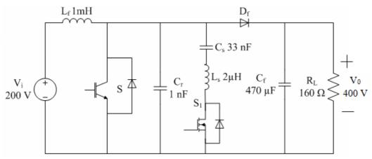
Figure 10. The model of ZVZCT Converter-I used in simulation [7]
