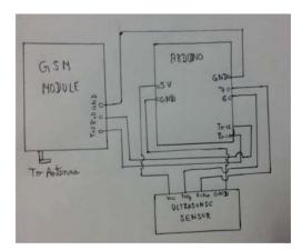
Fig 5: Circuit Diagram of Smart Waste System
