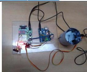
Fig. 12: SIM gets registered as the second red LED gets stop blinking.
