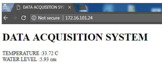
Fig. 10 Acquisition Result of Temperature & water level
