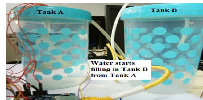
Fig.14 Status of tanks after water level exceeds
