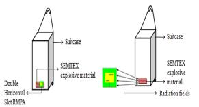
Figure 3.2 Proposed design to detect the SEMTEX materal
