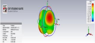
Figure 4.3 Directivity of double horizontal slot RMPA at 4.5GHz
