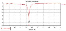
Figure 4.1 Return loss of double horizontal slot RMPA
