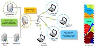
Fig. 5. The network-assisted adaptive video streaming testbed and the SOM map used in the WLAN AP's status classification [37].
