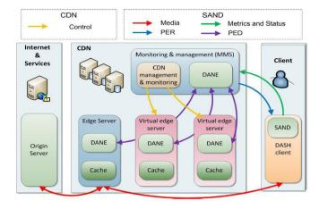
Fig. 9. Signaling in the advanced CDN architecture. [19].
