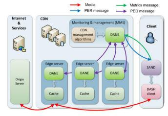
Fig. 4. Signaling in the advanced CDN architecture [49].
