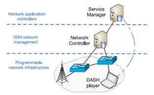
Fig. 8. DASH aware SDN architecture that separates data plane (network infrastructure) from control plane (network management and application controllers). The mixed-dashed line indicates a communication channel between DASH player and Service Manager [23].
