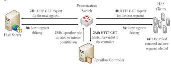
Fig. 6. Logical sequence diagram of the proposed solution [40].
