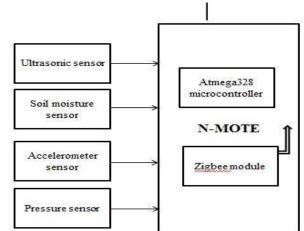
Fig 1. Transmitter Circuit.
