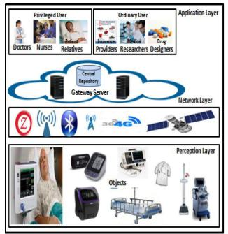
Fig.2 Architecture of smart healthcare system
