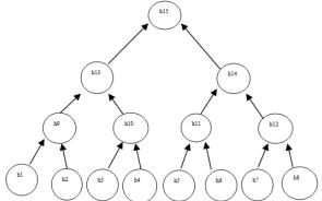
Fig 2. Applying Hash Functions
