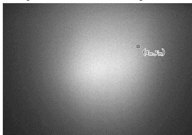
Fig. 2. TAOTF spectral image (635 nm) of the tungsten plate in vacuum under LH. Laser power is 8 W
