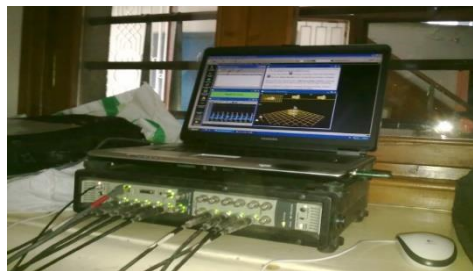
Fig. 6. Data acquisition system and the connection cables
