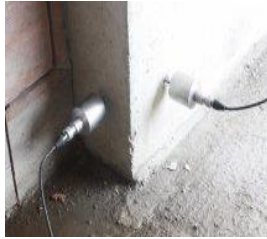
a) Mounting of the accelerometers
