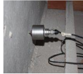
b) Mounting of reference accelerometer
