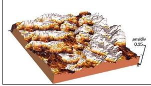
0.5% NaOCI- 10mins Fig. 1: AFM- dimensional change with 0.5% NaOCI with different time intervals
