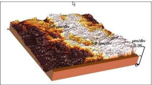
2.5% NaOCI- 10mins Fig. 2: AFM- images dimensional changes in 2.5% NaOCI at different time intervals
