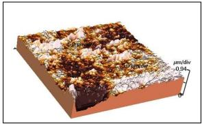
5.25% NaOCI- 10mins Fig. 3: AFM- images dimensional changes in 5.25% NaOCI at different time intervals
