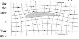
In the given figure of the aerofoil we can see that at some place the equipotential line and the stream line there is some concave portion so as a result there is a possibility of having a point of inflection. So, this can be determined by the following inequalities.
