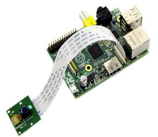
Figure3: Pi Camera Connection on Raspberry Pi
