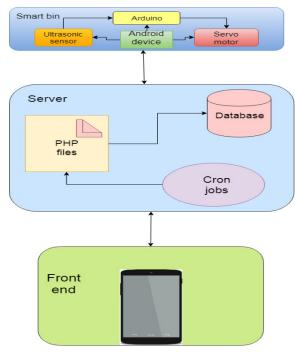
Fig 2: System Architecture
