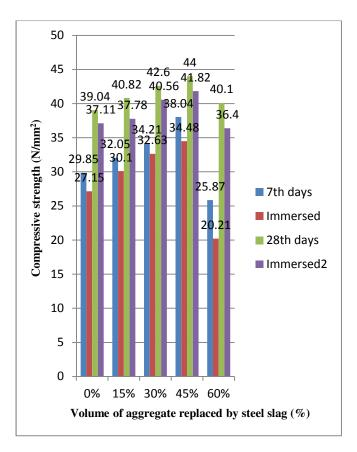
The Resistance to sulphate attack of concrete mix increases upto 16% if 45% of aggregate is replaced by steel slag at 28 days.
