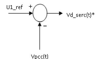
Figure 5. Series compensator controller
