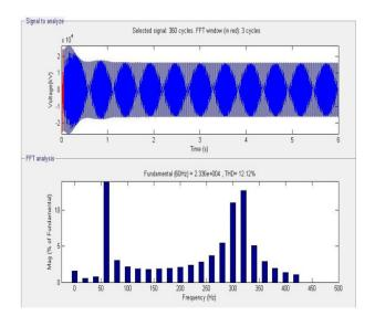
Fig.9. Result Of power system without UPQC
