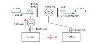
Fig (2): Block diagram of UPQC
