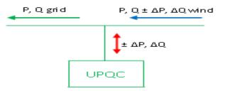
Figure 7. Power buffer concept
