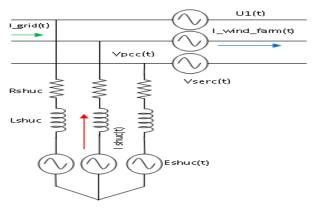
Figure 4. Power stage compensator model. AC side
