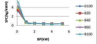
Fig 3(b): Variation of specific fuel consumption with BP with EGR
