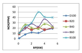
Fig -7(a): Variation of NOx with brake power without EGR
