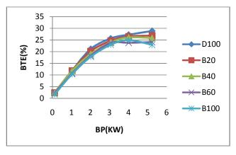
Fig -2(a): Variation of brake thermal efficiency with brake power without EGR
