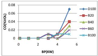
Fig -5(a): Variation of carbon monoxide with brake power without EGR
