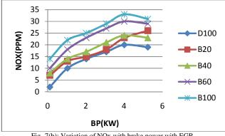
Fig -7(b): Variation of NOx with brake power with EGR
