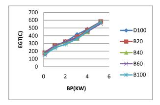
Fig -4(a): Variation of exhaust gas temperature with brake Power without EGR
