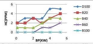
Fig -6(a): Variation of hydrocarbon with brake power and without EGR.
