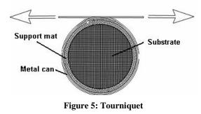
The tourniquet method is a fixed force, single seam method. The substrate is sleeved with a support mat and then inserted into rolled steel sheet and the closed by pulling on the opposite sides of the steel sheet until the set force is met and welded shut [6].
