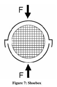
The shoebox canning method uses two prefabricated stamped out metal halves that are pressed with a fixed force to obtain the required GBD as in figure 5. The overlapped shell is then welded into place. The difference from the clamshell method is the overlapping of the halves.
