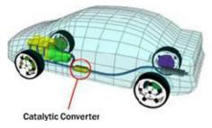
Figure 1: Catalytic Converter
