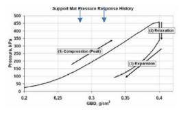
Figure 12: Mat pressure during compression [9]
