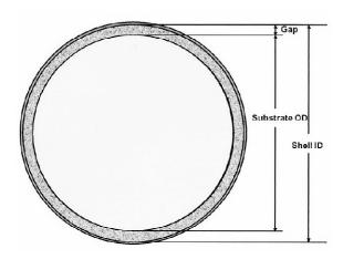
Figure 10: Intersection of Canned Substrate
