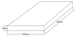
Fig. 1 Geometry of two way slab
