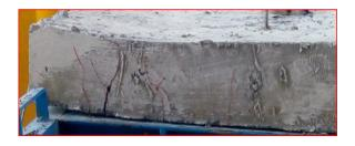
Fig.9 Corner uplift of CON slab
