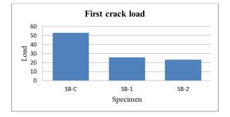
Fig. 12Bar chart representing first crack load of different specimen
