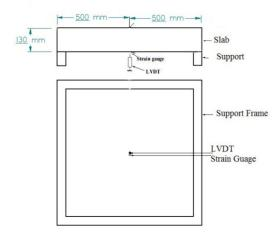
Fig. 4 Schematic diagram of test set up
