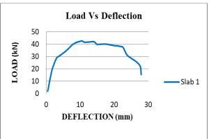
Fig. 7 Load vs. deflection graph for SB-1
