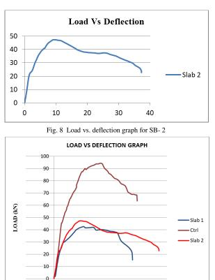
Fig. 9 Load vs. deflection comparison graph
