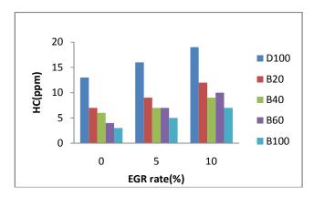
Fig -7: Variation of hydrocarbon with EGR.
