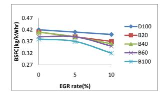
Fig -4: Variation of specific fuel consumption with EGR
