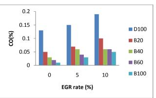
Fig.6: Variation of carbon monoxide with EGR. Fig.6 shows the variation of carbon monoxide emission with EGR at full load for diesel and blends of corn oil biodiesel. The CO emission depends upon the strength of the mixture, availability of oxygen and viscosity of
