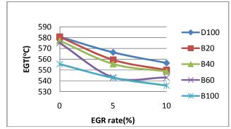
Fig -5: Variation of exhaust gas temperature with EGR.
