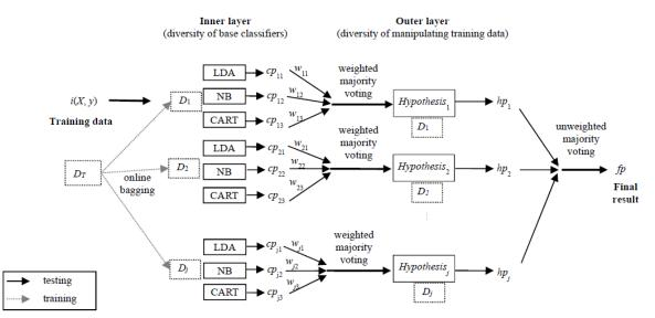
Fig 1. Illustration of Stage 1 in the MDDD.
