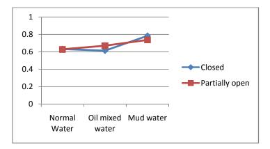
GRAPH 2: DISCHARGE FOR DIFFERENT TYPES OF WATER WITH RESPECT TO VALVE
