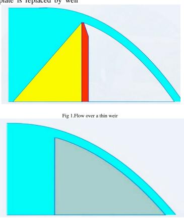
Fig 2.The fluid boundary bottom nappe has been replaced by solid boundary
