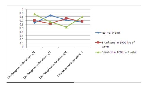
GRAPH3: BETWEEN COEFFICIENTS OF DISCHARGE FOR DIFFERENT WATER PERCENTAGE
