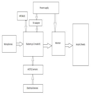
Fig 2. Smart mirror block diagram.
