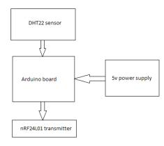
Fig 1. Temperature and humidity data source block diagram.
