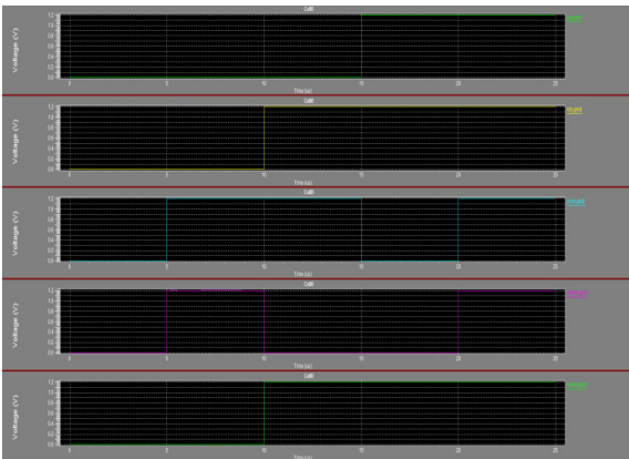
Fig.6. W-edit output waveform of 8T full adder
