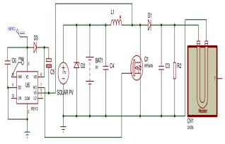
Fig. 2: Circuit diagram of a microcontroller based automated incubator
