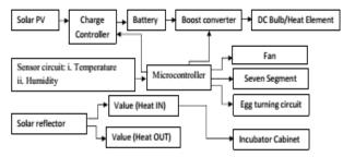
Fig. 1: Block diagram of a solar powered automated incubator for chickens
