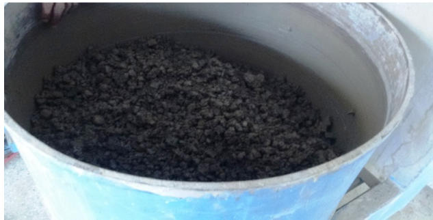
Fig.5 Concrete mixture after replacement by scrap rubber
