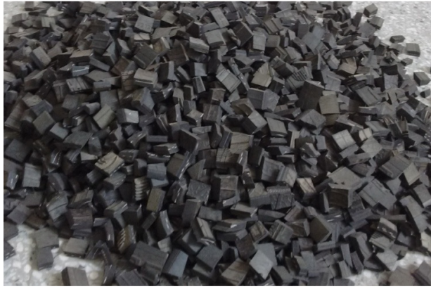
Fig. 4 Size and shape of rubber aggregate
