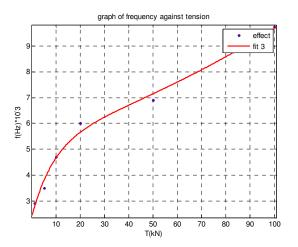
Figure 11: Graph of frequency against tension in transverse direction based on 30kg/m
