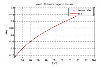
Figure 10: Graph of frequency against tension in transverse direction
