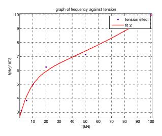
Figure 9: Graph of frequency against tension in normal direction
