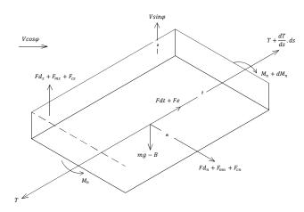
Figure 3: Forces and moments acting on a cable element
