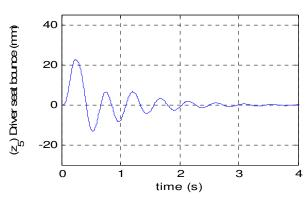
Fig.5 Driver bounce at 25 km/h speed.
