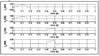
Fig.4 Wheels bounce at 25 km/h speed.
