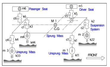
Fig.1 A Simplified Physical Model of the Vehicle
