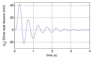
Fig.6 Driver bounce at 50 km/h speed.
