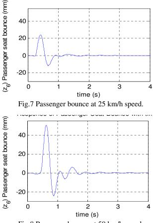
Fig.8 Passenger bounce at 50 km/h speed.
