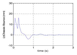
Fig.10 Chassis bounce at 50 km/h speed.
