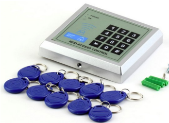
Figure 6.6: Access Control System
