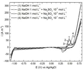
Figure 3. Cyclic voltammograms recorded on Ni–Pt NPs electrode in 1 mol L<sup>-1</sup> NaOH solution without and with different sulphite concentrations, at 5 mV s<sup>-1</sup>.
