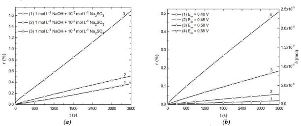
Figure 7. Chronocoulometric curves for Ni–Pt NPs electrode in 1 mol L<sup>-1</sup> NaOH solution with different sulphite concentrations, at  $E_{0x}$ =+0.55 V (*a*) and in 1 mol L<sup>-1</sup> NaOH + 10<sup>-1</sup> mol L<sup>-1</sup> Na<sub>2</sub>SO<sub>3</sub> solution (*b*).
