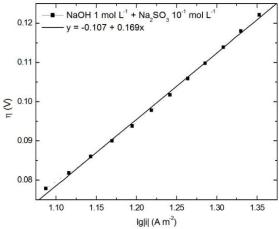
Figure 5. Tafel plot for sulphite oxidation on Ni–Pt NPs electrode in alkaline solution with  $10^{-1}$  mol L<sup>-1</sup> sodium sulphite.
