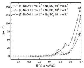
Figure 4. Linear voltammograms recorded on Ni–Pt NPs electrode in 1 mol L<sup>-1</sup> NaOH solution with different sulphite concentrations, at 1 mV s<sup>-1</sup>.
