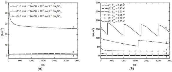
Figure 6. Current-time curves for Ni – Pt NPs electrode in 1 mol L<sup>-1</sup> NaOH solution with different sulphite concentrations, at  $E_{ox}$  = +0.55 V (*a*) and in 1 mol L<sup>-1</sup> NaOH + 10<sup>-1</sup> mol L<sup>-1</sup> Na<sub>2</sub>SO<sub>3</sub> solution (*b*).
