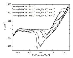
Figure 1. Cyclic voltammograms recorded on Ni – Pt NPs electrode in 1 mol L<sup>-1</sup> NaOH solution without and with different sulphite concentrations, at 500 mV s<sup>-1</sup>.
