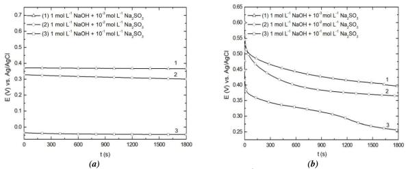
Figure 8. OCP curves for Ni–Pt NPs electrode in 1 mol L<sup>-1</sup> NaOH solution with different sulphite concentration before (a) and after (b) oxidation.
