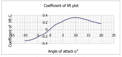
Figure 8. Coefficient of lift plot
