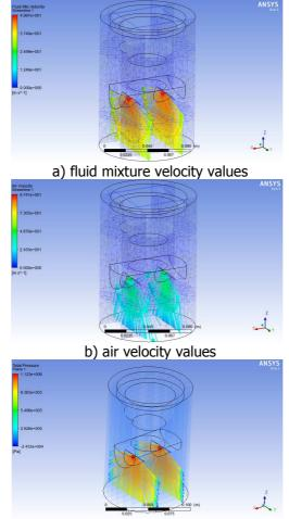
c) Total pressure values **Figure 5.** The obtained results for nozzle valve (model 1) The obtained results for nozzle model 2 (case 2) are presented in figure 6, in terms of fluid values and total pressure.
