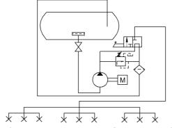
Figure 1. Schematic representation of sprayer installation components
