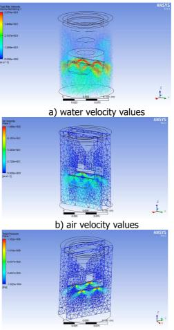
c) Total pressure values **Figure 6.** The obtained results for nozzle valve (model 2) The numerical results recorded on the two nozzle models (case 1 and case 2) are shown in table 1.
