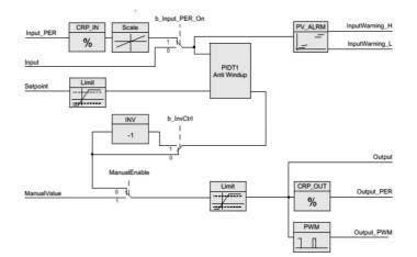
Figure 2. PID\_Compact – the block diagram
