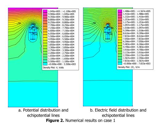
From the above figure can be observed an increasing of electric potential in the high part of the head human. The lowest values of electric potential can be founded near the ground (where was considerate as a reference one. The distribution of electric potential is a symmetrical one beside a middle line of the domain field considerate.
