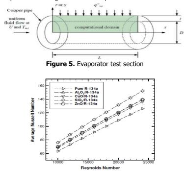
**Figure 6.** The effect of nanorefrigerant types on the average Nusselt number (Using  $\phi = 4\%$ , dp = 20 nm and qw = 5000 W/m2).
