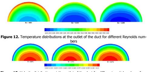
Figure 13. Velocity distributions at the outlet of the duct for different particle volume fraction
