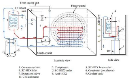
Figure1. Schematic arrangement of the experimental set-up
