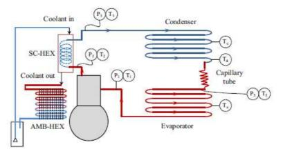
Figure 3. Location of temperature and pressure measurement in the experiment
