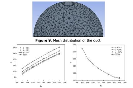
**Figure 10.** The changing of (a) average heat transfer coefficient and (b) average Darcy friction factor; with Reynolds number for different particle volume fractions
