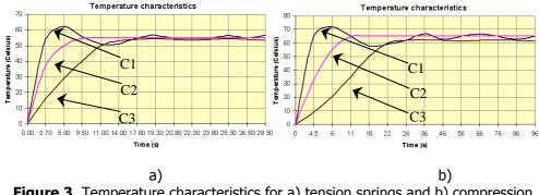
Figure 3. Temperature characteristics for a) tension springs and b) compression springs
