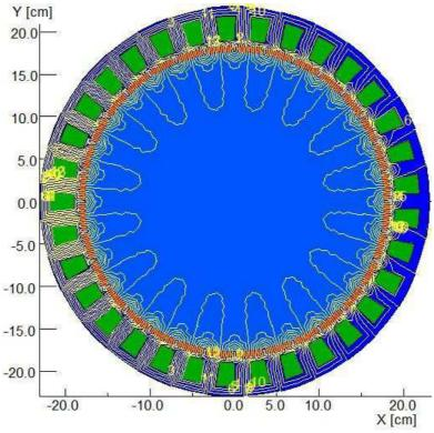
Figure 8. Magnetic potential field lines – case 3.
