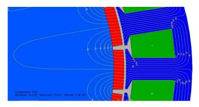
**Figure 11.** Magnetic induction field lines when the magnet is placed with the "d" axis perpendicularly to the stator tooth.
