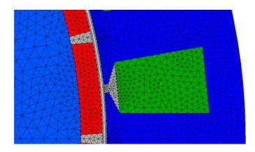
Figure 3.b. Discretization mesh – case 1.
