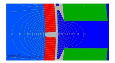
Figure 9.a. Magnetic induction field lines.
