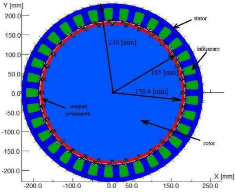
Figure 1.a. Generator typology and its main geometric dimensions.
