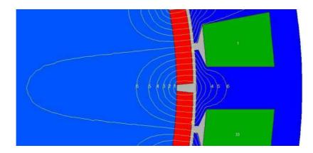
Figure 4.b. Magnetic potential field lines for case 1.
