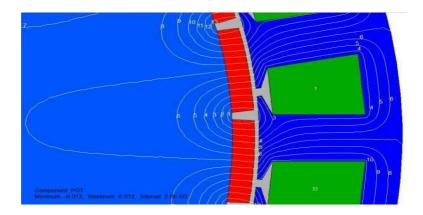
**Figure 10.** Magnetic induction field lines after the rotor rotation by a pole pitch quarter.
