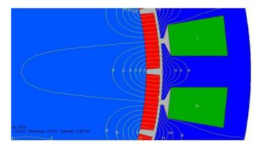
Figure 9.b. Magnetic induction field lines.
