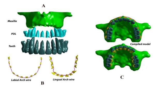
Then the constructed model was exported to the FE software ANSYS 12.0 (Swanson Analysis Co., Houston, TX, USA). The elements and nodes in the FE model (bone, tooth, PDL, bracket, wire) are listed in Table I.
