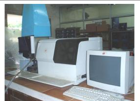
Fig. 3: Atomic absorption spectrophotometery Unit
