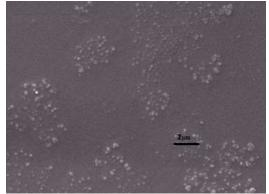
Fig. 1: Scanning electron microscopy result of BSA-EA-MWCNTs submicron hybrid nanocomposite
