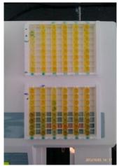
Fig. 5: Wells with stop solution
