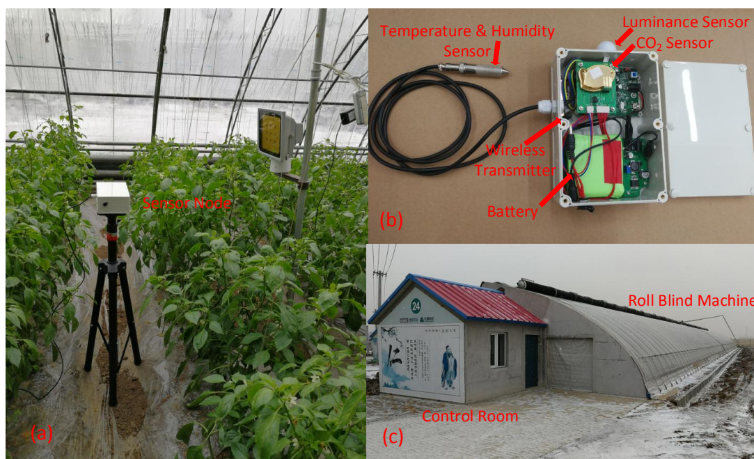
Fig. 3 - Photo of the sensor node working in the greenhouse (a), the inside view of the developed sensor node (b) and the outside view of the greenhouse (c)
