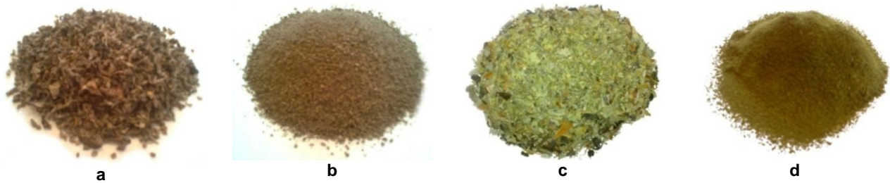
Fig. 2 - The plant material before and after grinding a,b – valerian root before and after grinding; c, d – gathered herbs before and after grinding
