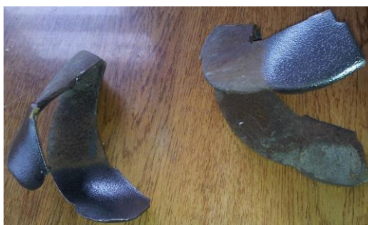
Fig. 2 – Corrosive damage of auger conveyor of agricultural materials
