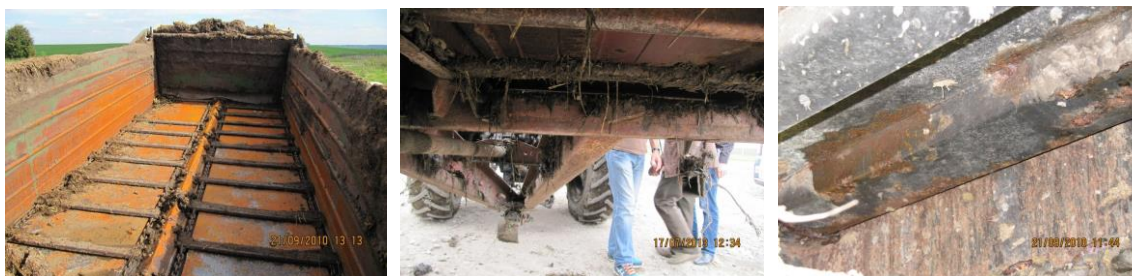
Fig. 1 – Corrosive damage of metal structure material of agricultural trailers
