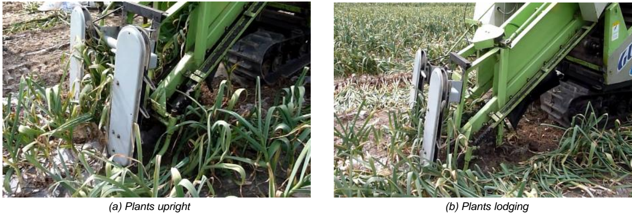
Fig. 5 - Working effect of the stalk lifting device
