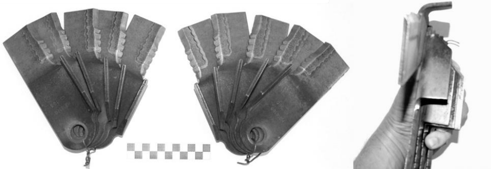
Fig. 2 - Set of experimental working elements for straw disperser of grain combine harvester "John Deere W650"
