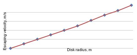
Fig. 5 - The dependence of granule escaping velocity on the disk radius
