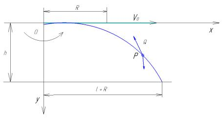
Fig. 6 - Diagram of granules flight analysis
