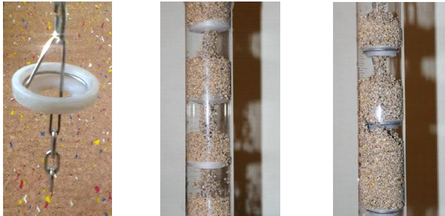
Fig.4 - A beaded operating element and the process of transporting and stirring of mixed fodder in a vertical route segment of a technological lane
